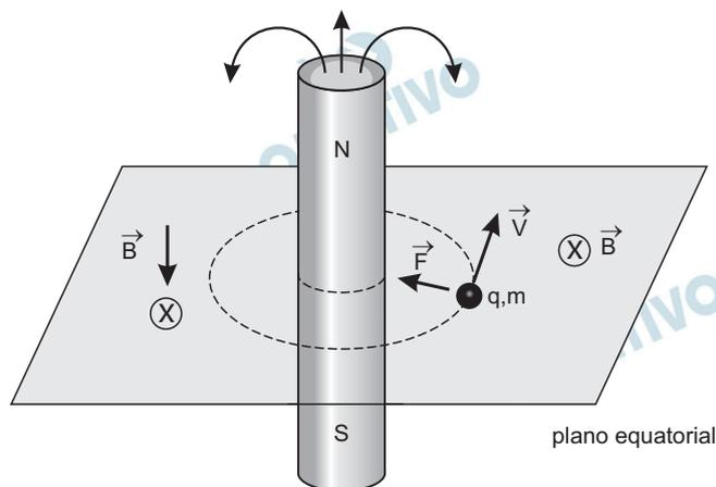
$$\left. \begin{aligned} F &= q \cdot v \cdot B \\ F &= \frac{m \cdot v^2}{R} \end{aligned} \right\} \frac{m \cdot v}{R} = q \cdot B$$
